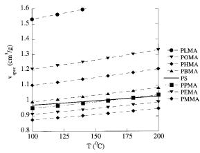
Figure 10. Calculated specific volumes of the different poly *n*-alkyl methacrylates and PS as a function of temperature.
