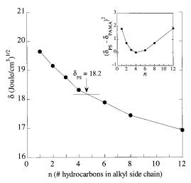
**Figure 9.** Calculated solubility parameters for poly *n*-alkyl methacrylates as a function of the no. of hydrocarbons *n* in the alkyl side chain. The value for PS is indicated by the vertical arrow. The inset represents the difference  $(\delta_{PS} - \delta_{PAMA})^2$  for each of the methacrylates.
