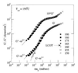
**Figure 6.** Master curves for the storage (G') and loss (G')moduli of 136K PS-b-PPMA.
