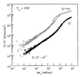
**Figure 1.** Master curves for the storage (G') and loss (G'')moduli of 45K PS-b-PLMA.
