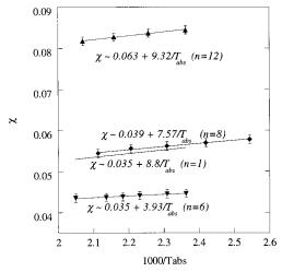
**Figure 5.** Segmental interaction parameters  $\gamma$  extracted from SANS data for 19K  $PS_{d8}$ -*b*-PLMA (n = no. of hydrocarbons in side chain = 12), 23K PS-b-POMA (n = 8) and 27K PS-b-PHMA (n = 6). Also shown is the interaction parameter for PS-*b*-PMMA (n = 1) listed in ref 28.
