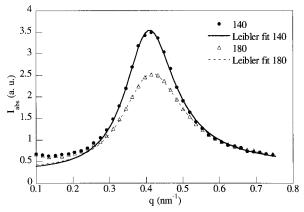
**Figure 4.** Scattering intensity profile for 23K PS-*b*-POMA at 140 °C and 180 °C and the corresponding Leibler fits.
